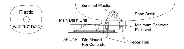
Step 2 (Option) Rather than using dirt to pack around the flange and pipe to restore the integrity of the pond bottom around the flange, again., you can use concrete just as effectively. Although a bit more trouble initially, concrete is very effective. It will not compress once water is added to the pond. When using concrete, excavate about 16" to 18" width for the drain
