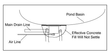
placement rather than 12". Also, finish with the flange plate and concrete about 3/8" below the dirt level of the pond bottom. This will allow for any settling of the existing dirt bottom under the weight of water to finish out at the poured concrete level.
