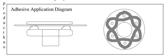
wn as LEXEL is an extremely dependable inexpensive adhesive for underwater applications such as drains.
