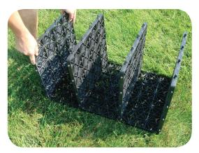
There are seven rows of holes for setting the support panels. Push the four end / center panels into place utilizing the two end positions and the two rows located on either side of the center position. Be sure you insert the long tabs at this stage leaving the short tabs facing to the sides.
