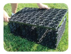
Place the second large side panel on top of the four support panels. Start at one end and work one complete row at a time into place making sure to keep everything aligned.
